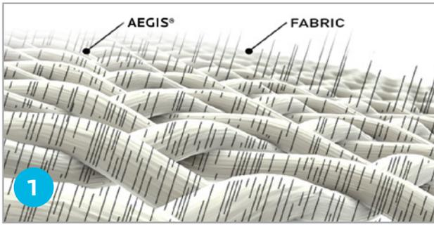
**AEGIS® IS BONDED TO THE FIBERS DURING MANUFACTURING.**
